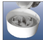
Pouring Replicast Around the Model
